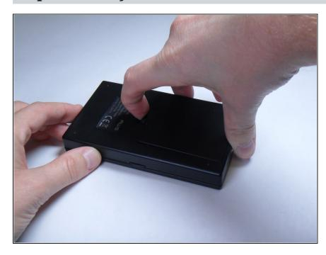
Use your finger to pull up on the battery cover tab and lift to remove.
