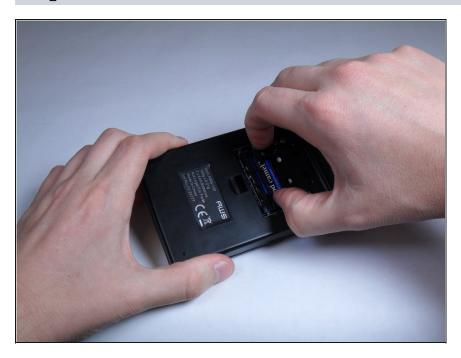
Use fingers to remove and replace both triple-A batteries.
