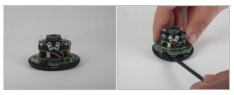
Insert a spudger tool under the micro-USB port and lift to separate the motherboard from the back case.
