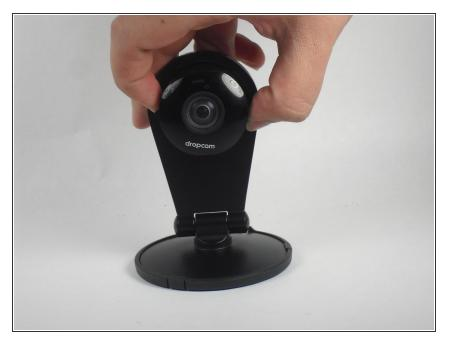
Press in the mounting clips on each side of the case to remove the camera from the mount.
