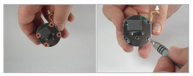
• Using a Philips #0 screwdriver, remove the four 2mm screws.
