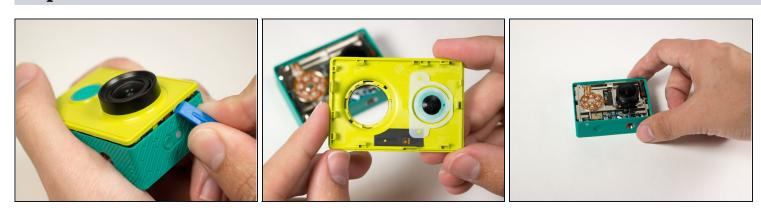
• Slide prying tool along the seam until front panel is fully separated from the back panel.
