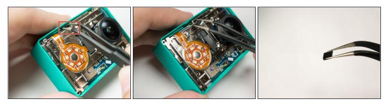
• Pull on and remove the black spacer located at the top inside of the camera body using the <u>tweezers</u> and set the part aside.
