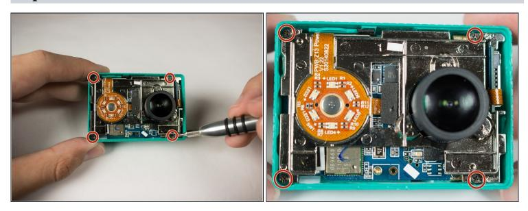
• Remove the four 3.8 mm Phillips #000 screws located in the outer corners of the motherboard.
