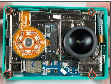
Remove the four 3.8 mm Phillips #000 screws located in the outer corners of the motherboard.
