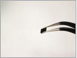
Pull on and remove the black spacer located at the top inside of the camera body using the tweezers and set the part aside.
