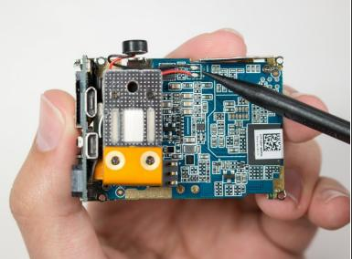
• Locate the solder points connected to the red and black wire on the back of the motherboard.
