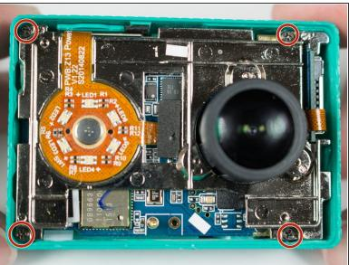
Remove the four 3.8 mm Phillips #000 screws located in the outer corners of the motherboard.
