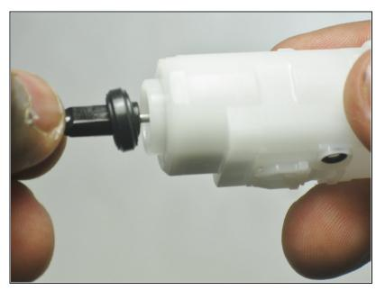
Remove the rubber stopper from the top of the motor shaft by gently pulling it off.
