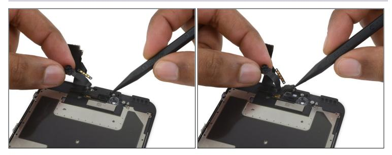
• Use the pointed tip of a spudger to lift the ambient light sensor from its housing in the front panel.
