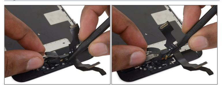
• Insert the pointed tip of a spudger between the microphone flex cable and the front panel to break the adhesive holding it in place.
