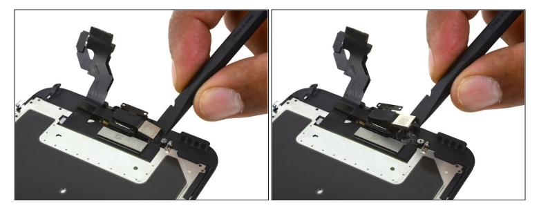
• Use the flat end of a spudger to lift the FaceTime camera out of its housing.
