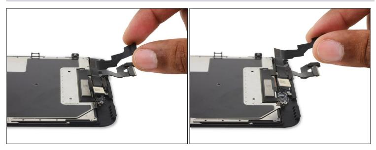
• Remove the FaceTime camera and sensor assembly.
