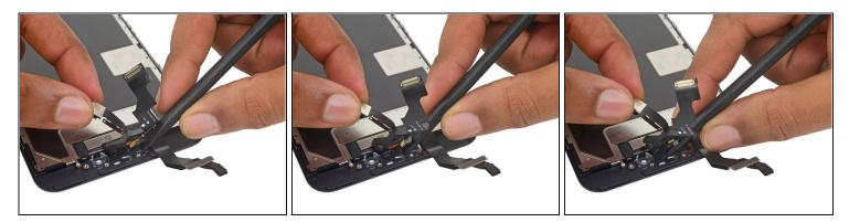
• Use the flat tip of a spudger to lift up the microphone and earpiece gasket.
