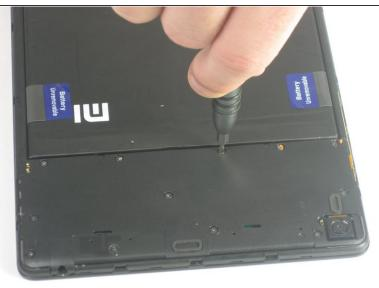
Remove the twelve 3.0 mm Phillips #000 screws on the upper cover of the device.
