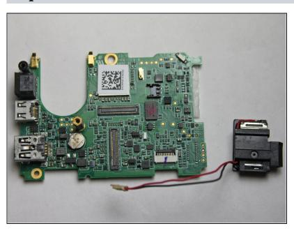
Once disconnected from the motherboard, the speaker assembly can be removed.
