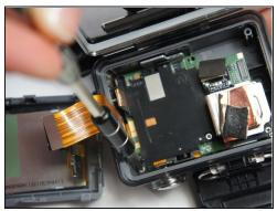
• Remove the three 4 mm Phillips #000 screws securing the motherboard.
