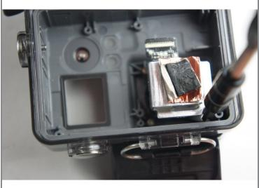
• Remove the four 4 mm Phillips #000 screws securing the lens to the case.
