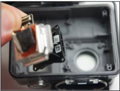
• Gently lift the lens up and out of the device.
