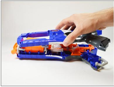
• First, remove the outer parts of the blaster, starting with the top part of the cocking mechanism. Then remove the full cover itself.
