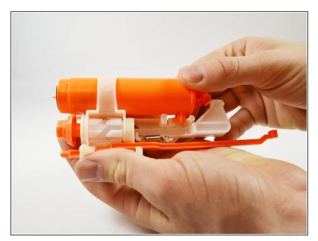
Remove the spring air compressor component.
