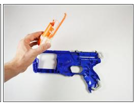
Remove the trigger, the cocking holdback, and the air compressor chamber
