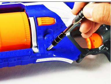
Locate the 12 Philips head screws and remove them: Head Diameter= 4.3mm, Thread Pitch= 1mm, Screw Length= 8mm
