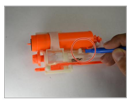
Remove the spring holding the air compressor together.
