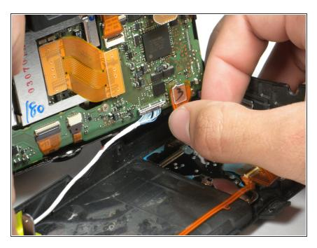
Disconnect the orange cable at the bottom of the camera by gently pinching with your fingers.
