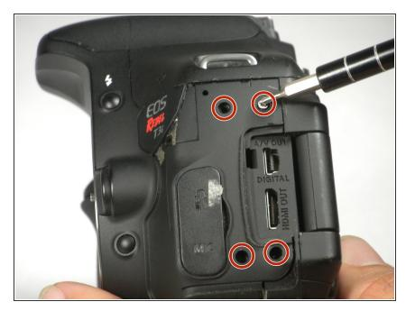
Remove four 3 mm Phillips #000 screws on the left side of the camera.
