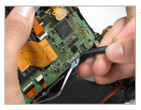
Detach the blue cable by sliding the pointed end of a spudger between the motherboard and the silver prongs connected to the cable.
