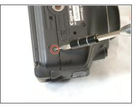
• Remove four 3 mm Phillips #000 screws on the bottom of the camera.
