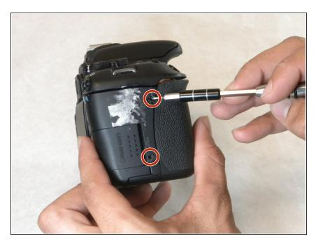
Remove two 3 mm Phillips #000 screws on the right side of the camera.
