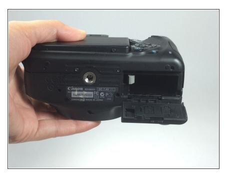
Remove the battery from the compartment.
