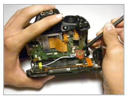
With the spudger, remove the orange ribbon cable leading to the circuit board from the back of the camera.
