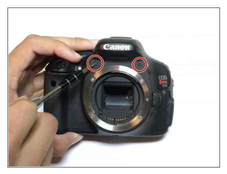
Remove the two 6 mm Phillips #000 screws.
