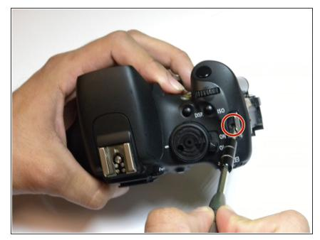
On the opposite end of the camera, unscrew the screw next to the power switch using the same tool.
