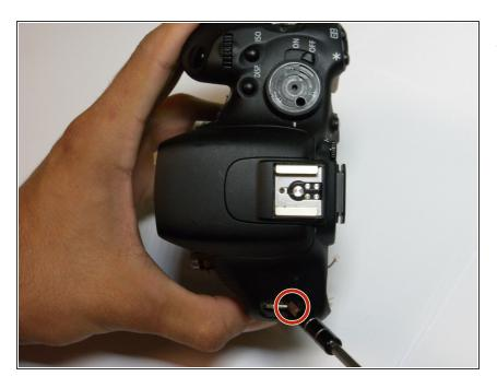
Remove the single 4 mm Phillips #000 screw located near the strap mount.
