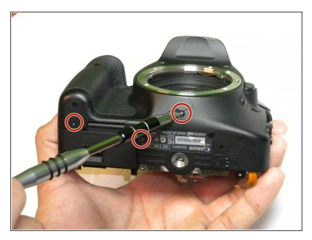
Remove the single 6 mm and two 3 mm Phillips #000 screws.
