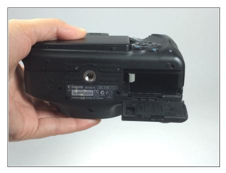
Remove the battery from the compartment.
