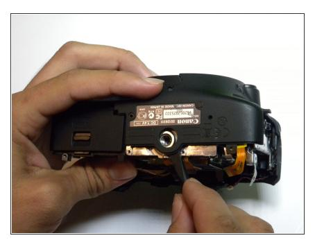
Use the spudger to lift the plastic under the tripod mount.
