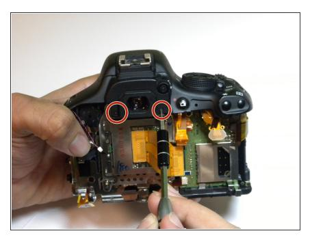
Remove the two 5 mm Phillips #000 screws.
