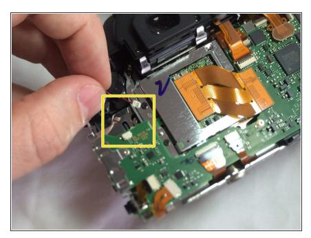
Disconnect this tiny plug. Make sure to only pull on the white plastic. You can use a dull single-sided razor blade to pry the white plastic connector from its base.
