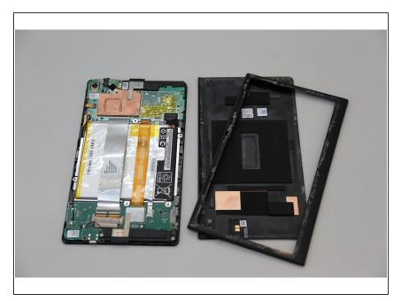
When you take the rear panel and the frame out, place the rear panel and the frame away from the device.
