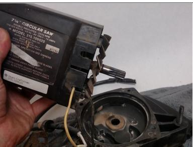
The motor will now be loose and you should be able to twist the motor in a counter-clockwise direction until it is able to be pulled off.
