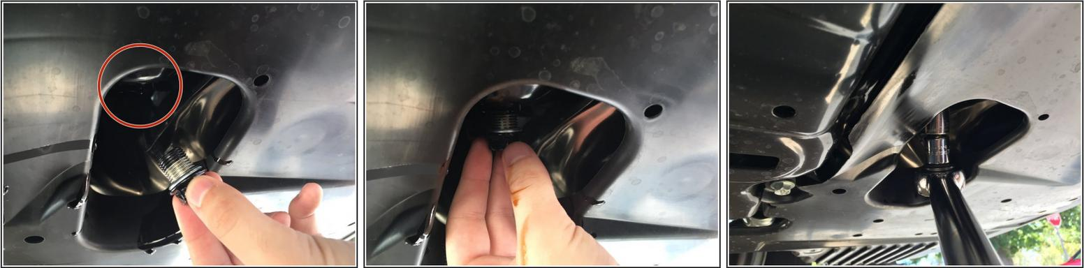
☑ When reinstalling the oil drain plug, replace the crush washer (part# 803916010) .
