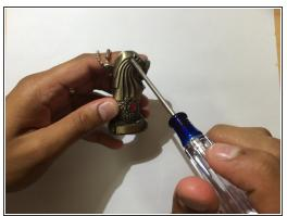
Use the screwdriver to remove all the 1.2 mm Phillips #1 countersunk screws from the torch.
