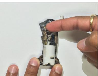
Gently bend the sparker until it is positioned near the opening of the Merlion's mouth.
