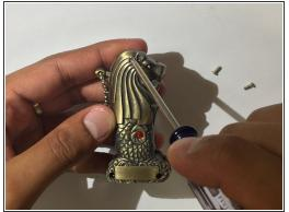
Use the screwdriver to put the screws back in the torch.
