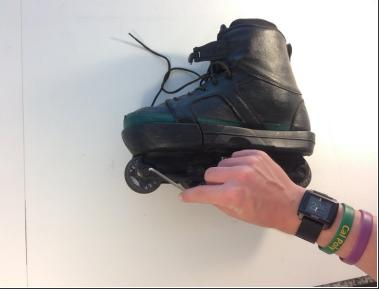
Remove the wheels with the allen wrench. All screws for the pictured boot require a 5/32 allen wrench and are 10mm long.
