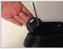
Flip the boot over, but be careful to hold the bolt into the frame. Add the 10mm screw to the hole and reattach it with the allen wrench.
