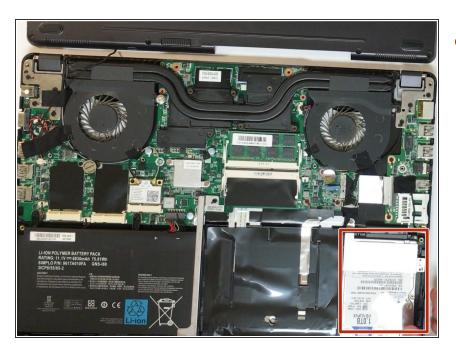
Locate hard drive in the bottom right of the laptop.
