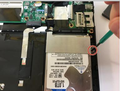
Remove the two screws holding the hard drive in the laptop.
