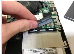
Remove the SATA connector by gently prying the far right, and then the far left of the connector until it slides out of the hard drive.
