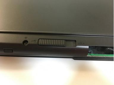
Slide the switch on the base of the laptop from locked to open.
