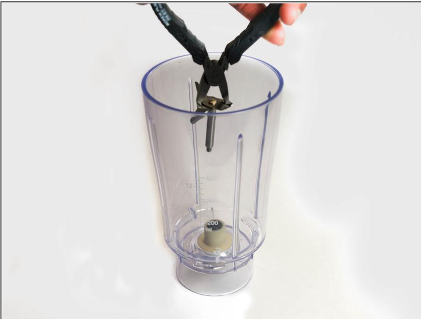
**⚠** Carefully, pull the blades out of the container as they are very sharp.
