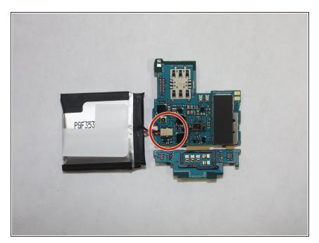
Once the motherboard and the battery are removed, disconnect the battery at the connector.
