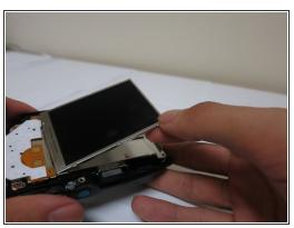
Slide the spudger under the LCD screen and pry it off. Since the screen is glued down with adhesive, some effort may be required.
