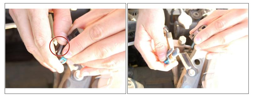
• Lift up on the latch and pull. The bulb will come free from the wires.
