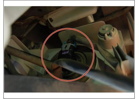
Locate the bulb. It will be in the front and to the side. Start with the side opposite from the battery.
