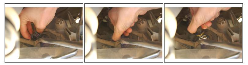
• Twist assembly 45 degrees counter clockwise and pull straight out.
