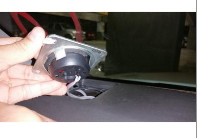
Gently lift the tweeter bracket with the tweeter inside and locate the connector.
