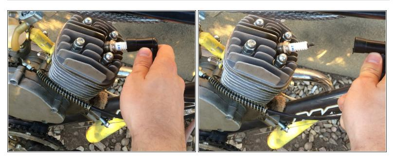
Detach the rubber CDI from the spark plug by gently pulling up and away from the engine.
