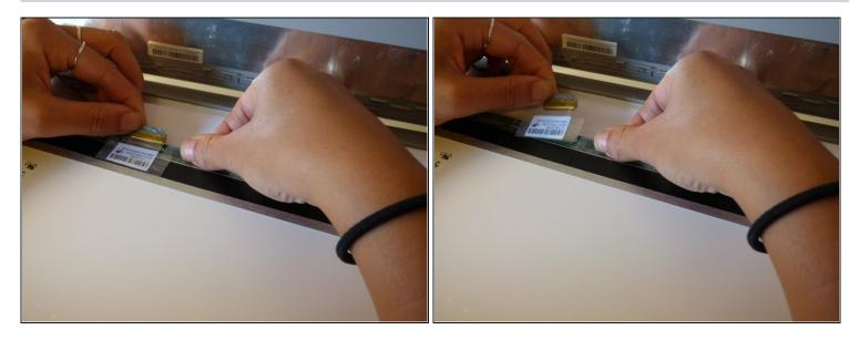
• Remove the video cable from the connector by gently pulling the gray tab out.
