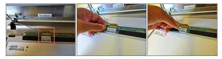
Gently peel off the bar code sticker that is connected to the video cable connector.
