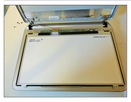
Now that the screen is not screwed in, place it face down on the keyboard.
