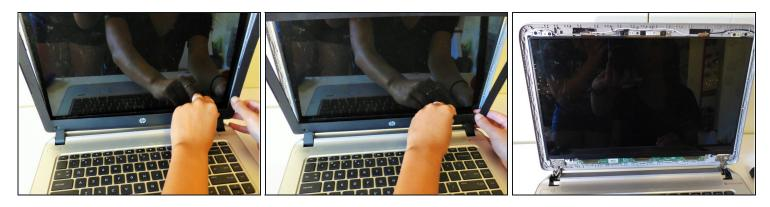
• Separate the border entirely by unsnapping the plastic snaps all the way around the screen until you can remove the border.
