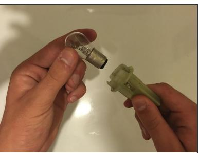
The 7528 bulb is in the off-white plastic carrier. Apply slight pressure downwards and twist counterclockwise to remove the bulb.
