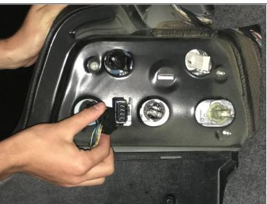
Pinch the top and bottom of the power connection. Pull hard on the power connection to remove it, disconnecting the wiring.
