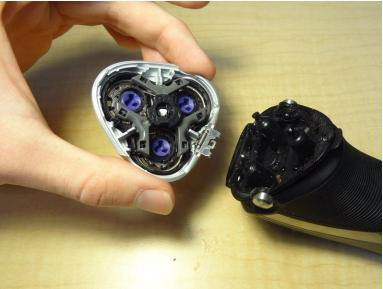
Grasp the sides of the head and pull straight up to detach it from the body.
