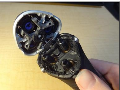
Begin by pressing the small button beneath the head to allow it to open.
