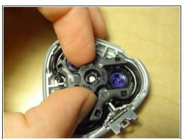
• Line up the locking mechanism with the new blades, then rotate the center clockwise to lock down.
