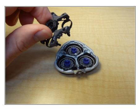
Lift the locking mechanism straight up, freeing the blades.
