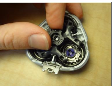
To unlock, rotate the center locking mechanism counter-clockwise.
