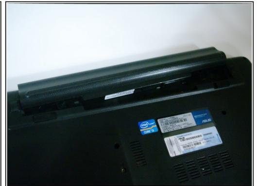
**⚠** Make sure the laptop is unplugged before removing the battery to avoid risk of electric shock.
