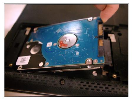
Gently slide the hard drive left toward the edge of the laptop, then lift up to remove it.
