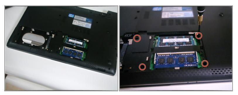
Remove the 4 Phillips #00 screws around the RAM.
