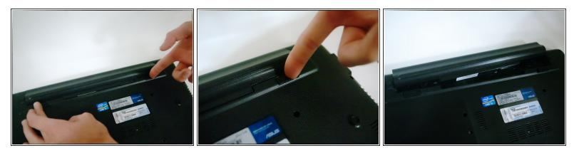
Make sure the laptop is unplugged before removing the battery to avoid risk of electric shock.
