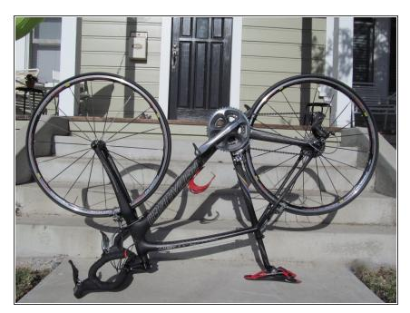
To easily remove the rear wheel, flip the bike upside down so that it's sitting on the handle bars and seat.
