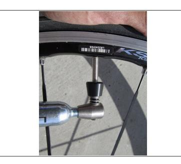
Now that the tire is back on the wheel, screw the adapter onto the CO2 cartridge and place it on the valve.
