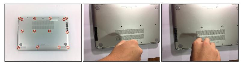
Use a Phillips screwdriver to remove the 14 screws securing the back cover.
