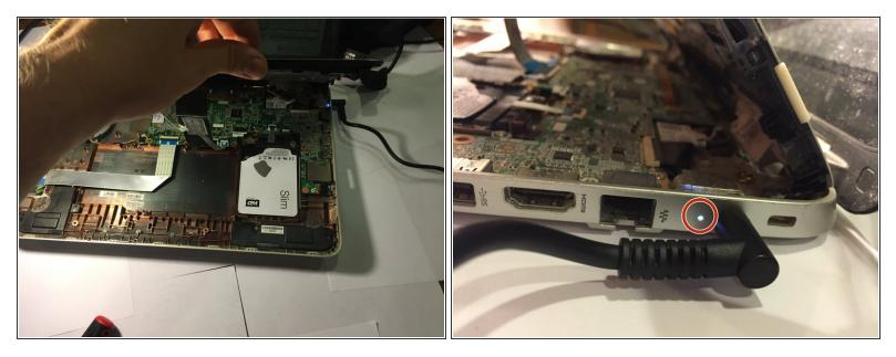
• Once the battery is safely removed, plug the charging cord into the charging port on the side and plug the other end into the wall.
