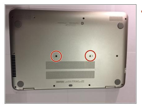
Flip the laptop over on its back and remove the two depressed stickers in the middle to reveal the two central 6.0 mm Phillips-head screws.
