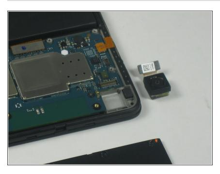
• Carefully remove the rear camera from the device.
