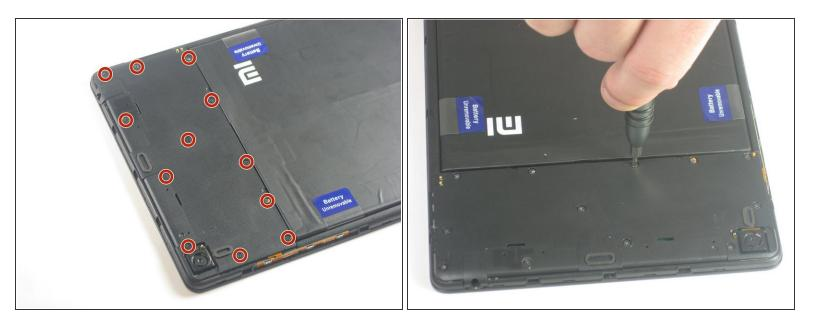
• Remove the twelve 3.0 mm Phillips #000 screws on the upper cover of the device.
