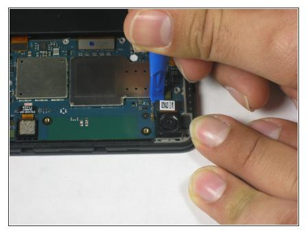
• Use a plastic opening tool to disconnect the rear-facing camera from the motherboard.
