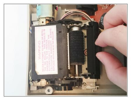
Remove the ink cartridge by pushing the tab back then lifting it out to gain access to the screw that holds the printer in place.
