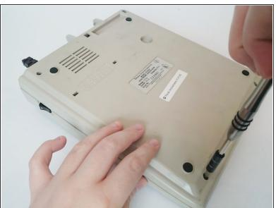
Flip the calculator over and remove the 4 main 10mm screws with a PH1 screwdriver.
