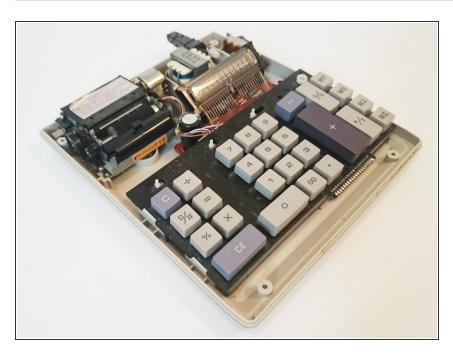
Flip the calculator back over and remove the top cover.
