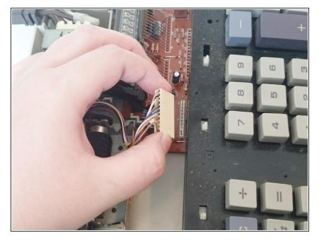
Disconnect the printing unit from the motherboard by pulling up on the connector – located in the bottom left of the motherboard.
