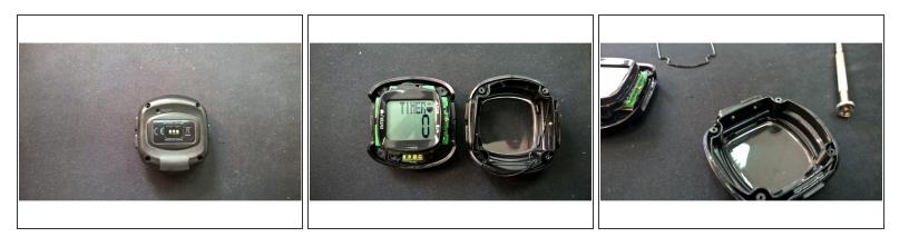
Remove 4 screws in corners from the back. Remove the cover. Thin silicone washer is visible now. The buttons look waterproof.
