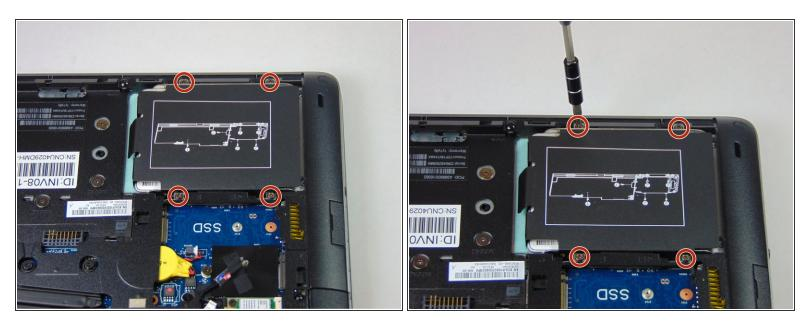
Loosen the four Phillips screws securing the hard drive.
