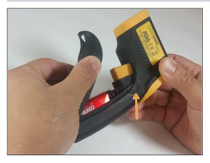
Pull the battery cover away from the handle by gripping near the thumb groove.
