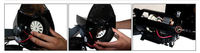
• Remove the motor compartment from the juicer and it is ready to be replaced.
