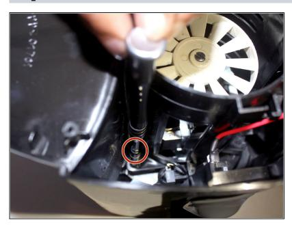
Unscrew the 19.1 mm screws inside the juicer holding the motor compartment attached to the juicer. Use the 2.5 mm Flathead adapter as the screw driver. The diameter of the screw head is 7.1 mm.
