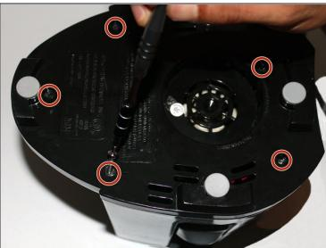
• Use the <u>2.5 mm Flathead</u> adapter to remove the 13.5 mm screws from the bottom of the juicer. The screw head diameter is 5.2 mm.
