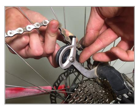
While temporarily lifting the chain off the pulley, check to see if the pulley rotates freely.
