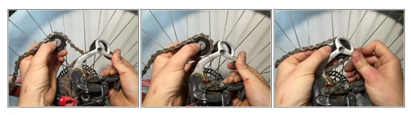
Place the teeth of the pulley against the chain, then push it with the chain into the derailleur arm.
