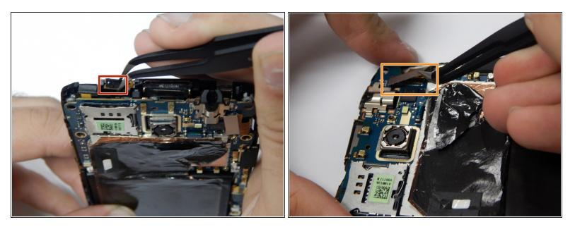
Use tweezers to disconnect the power button flex cable.
