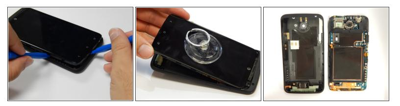
• Using plastic opening tools, pry open the bottom of the device first.
