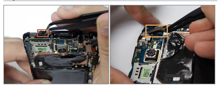
• Use <u>tweezers</u> to disconnect the power button flex cable.
