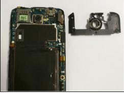
• Using a Philips head screw driver, remove the five 2.4mm screws that are pictured. Then remove the plastic cover.
