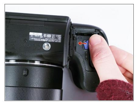
Push the blue tab that secures the battery. The battery will then spring out.
