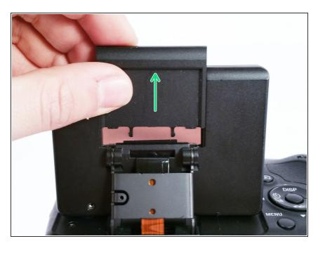
Remove the plastic cover from the back of the LCD display by simply sliding it up and off of the camera.
