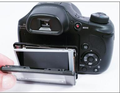
Using a plastic opening tool, carefully remove the plastic housing that surrounds the LCD display.
