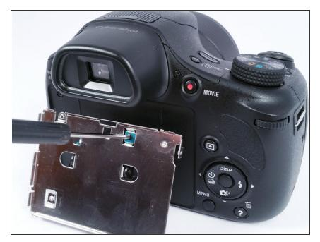
Using a small Phillips head screwdriver, remove the last 2 cm screw that mounts the circuit board to the metal LCD display frame.
