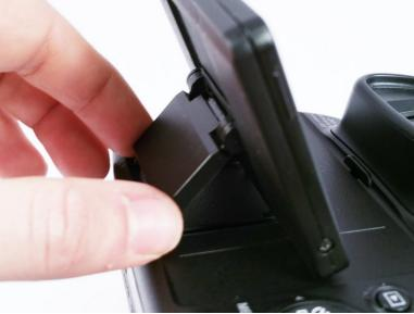
While using a plastic opening tool, carefully remove the plastic housing that surrounds the hinge.
