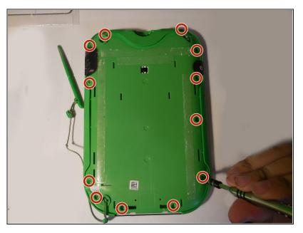
Remove the 7 mm screw to the right of the cartridge dock, two 8 mm screws in the top left, and the nine 8 mm screws holding the the green shell.
