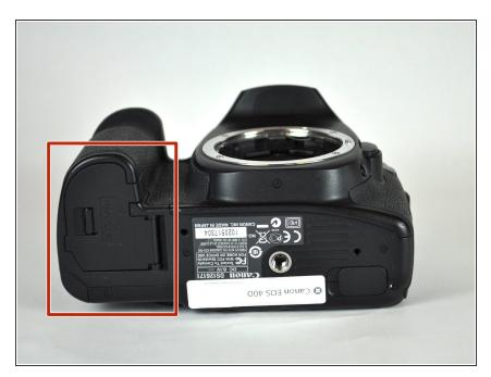
Locate the battery compartment cover on the bottom of the camera below the shutter button.
