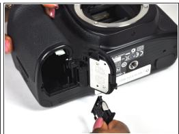
Remove the date and time battery holder by sliding it out of the slot.
