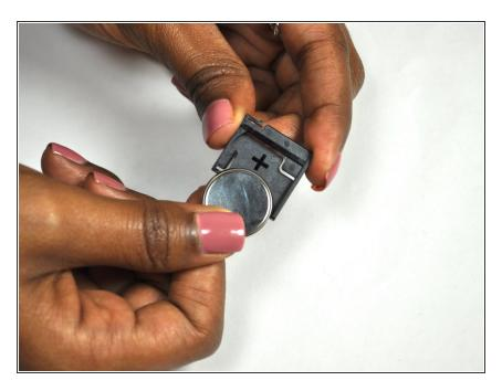
Remove the date and time battery from the battery holder.
