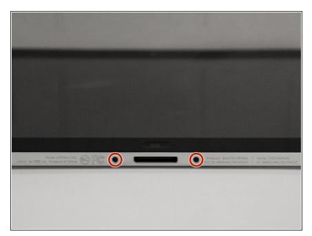
Unscrew the two 2.8mm Phillips #000 screws near the power connector.
