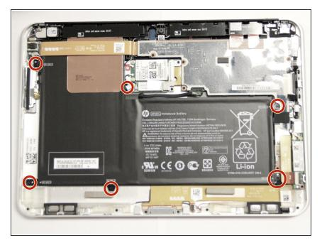
Remove the six 2.2mm Phillips #000 screws securing the battery to the device.
