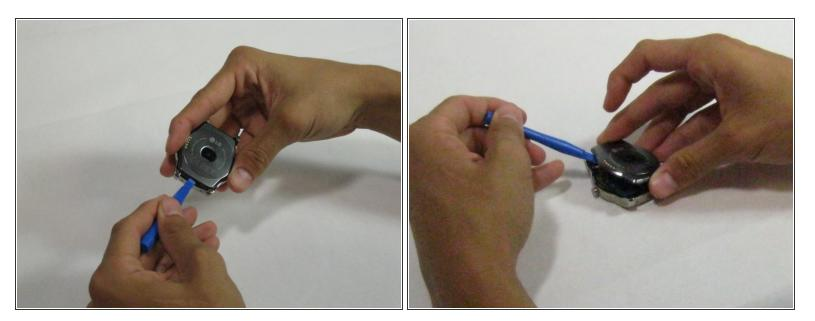
Using plastic opening tools, carefully pry open the back cover of the the watch.
