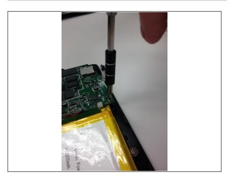
• Use a 4.0 bit screwdriver to remove the screws from the chip
