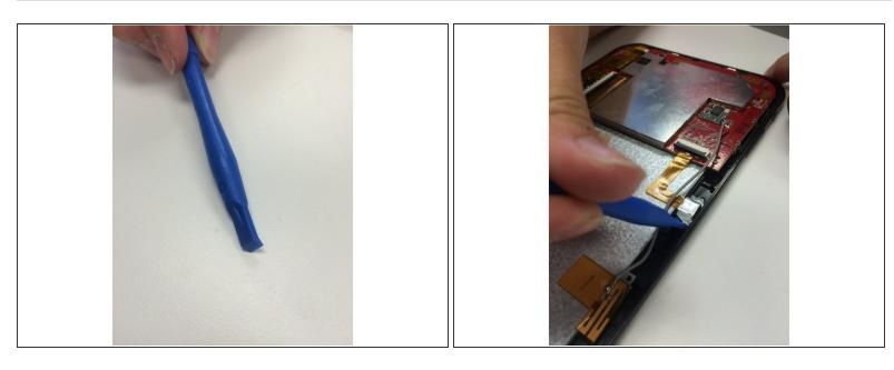
Remove silver foil from the back of the camera using the blue opening tool
