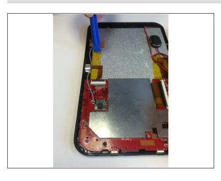
Remove yellow tape that is securing the camera wires
