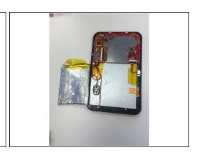
Pry battery away from the back of the tablet until the battery is completely separated from the adhesive
